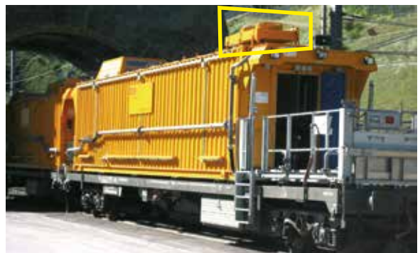
Radiator mounted separately on wagon roof
